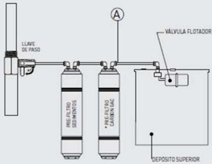
ESQUEMA HIDRÁULICO MODELO UF
